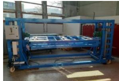
Handling and positioning tool for integration & tests
