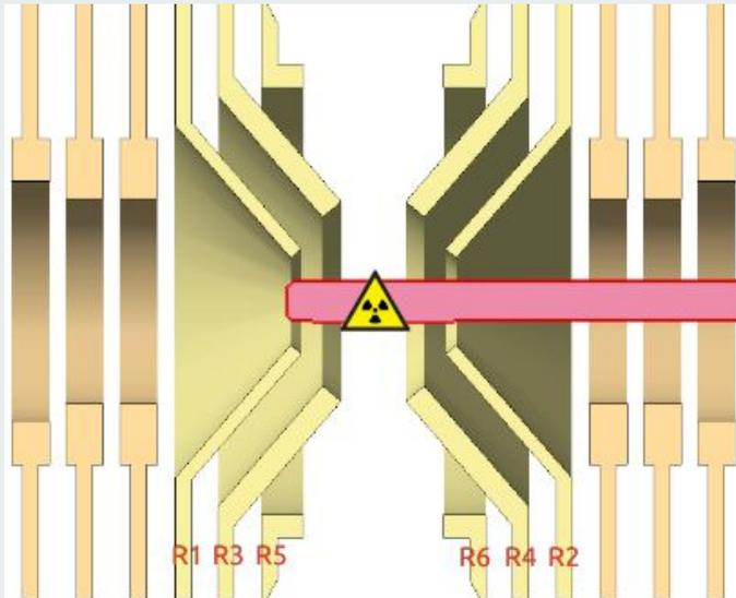
Paul Trap consisting on 3 pairs of **electrodes** (R1-R6) and 2 **Einzel lenses**
