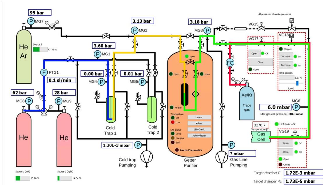
Injection of He + CF<sub>4</sub> gas (~10ppm), flow mass monitor
