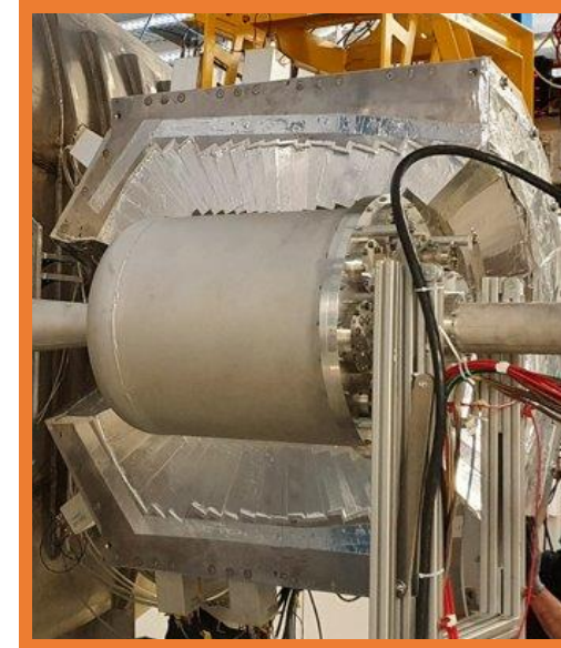
CALIFA ( \theta, \phi, \Delta E ) Array of CsI crystals
