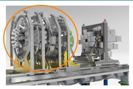
• The most forward polar angles  $(1.4^{\circ} < \theta < 12.6^{\circ})$  have been covered with 12 FAZIA blocks in a wall configuration at 1 m from the target. The first five rings of INDRA have been removed.
