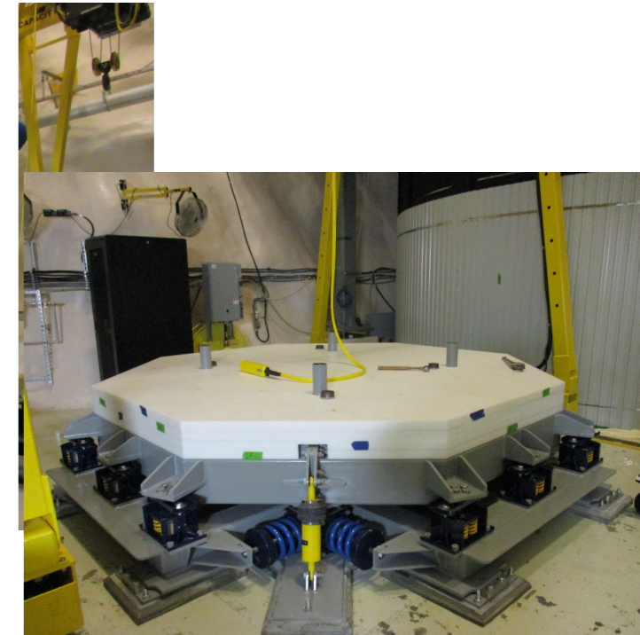
Seismic platform installation
