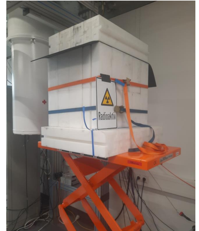
Portable neutron source near a dry cryostat ( < 7\text{mK} ) @ TUM
