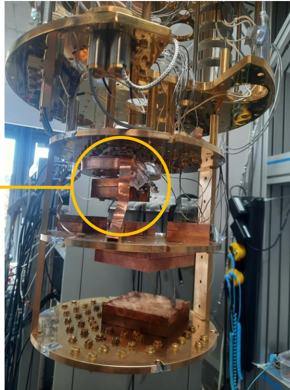
Two-stage spiral spring decoupling between assembly and detector holder
