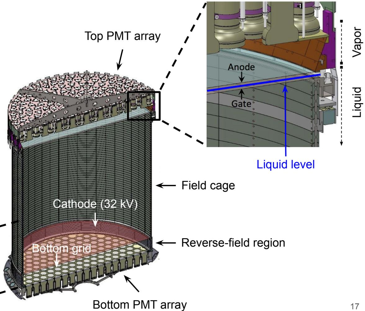
X,Y calculated from localized S2 light pattern in top photomultiplier tubes (PMTs)
