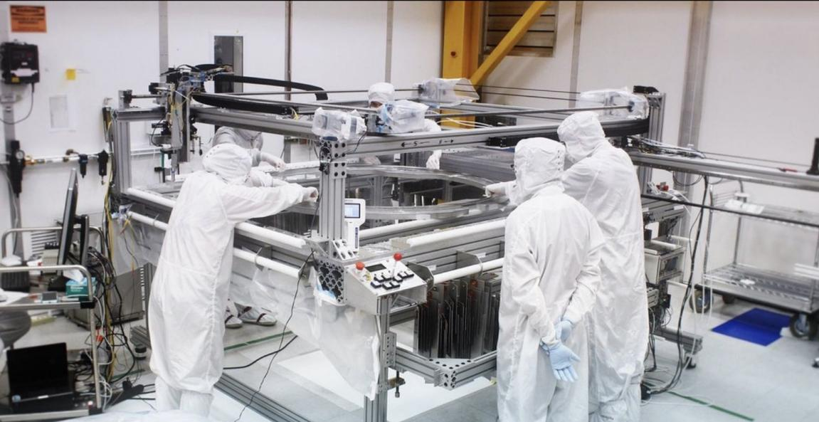
At SLAC, woven in custom loom, precise tensioning of wires, limit deflection of wires in electric field
