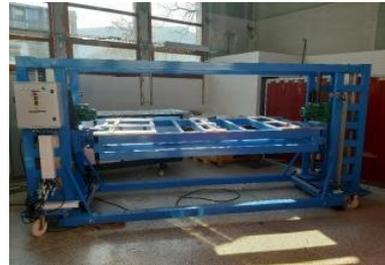
Handling and positioning tool for integration & tests
