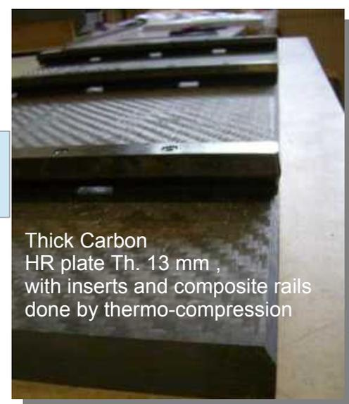
Thick Carbon HR plate Th. 13 mm, with inserts and composite rails done by thermo-compression
