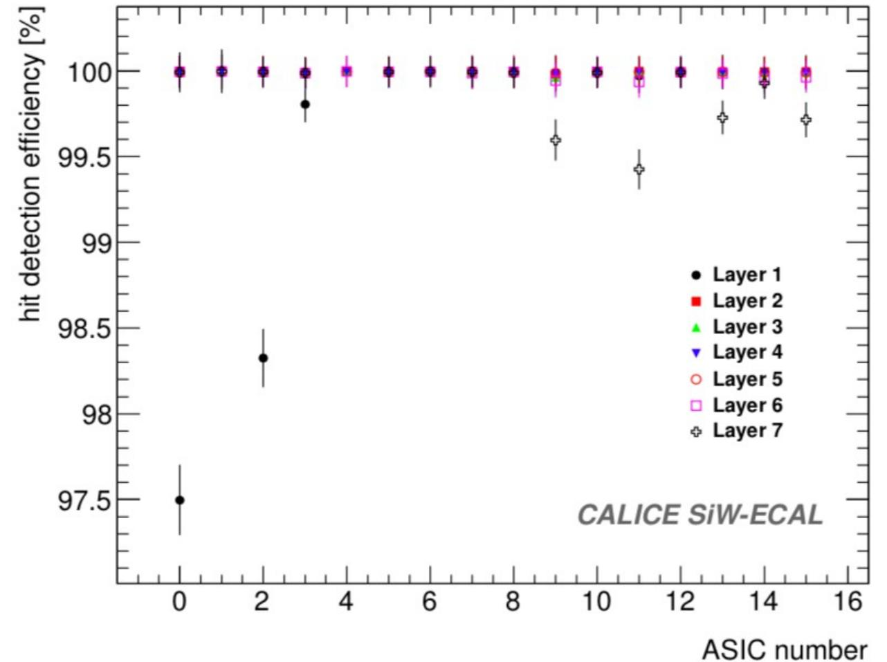
Trigger thresholds uniform at around 1/2 MIP
