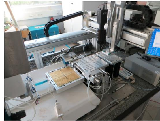
Wafer Gluing with robot
