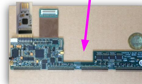
SL Board design is adapted to Heat exchanger geometry
