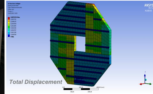
CFRP structures / End-Cap module : thick plates with inserts & longest layer : 3 alveoli L = 2.5 m wall thick. = 0.5mm
