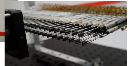
Fiber positioner "Cobra"
