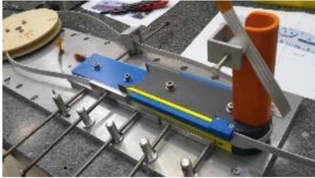
Winding mockups (test state of the art cables in prototype coils)
