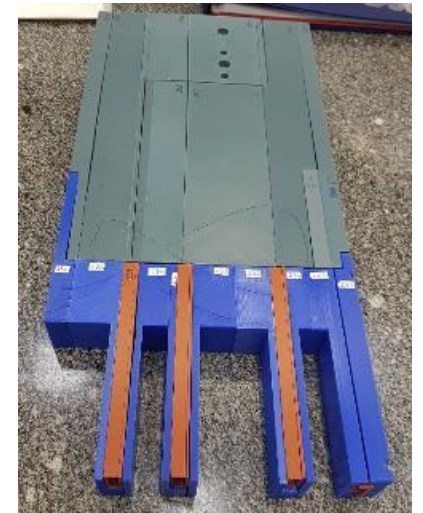
Joints mockups (test the grading technology before implementing it into coils)
