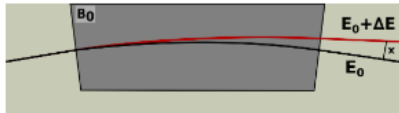
Figure 1: Dipole before tapering. A particle with an energy deviation \Delta E is forced away from the ideal orbit.
