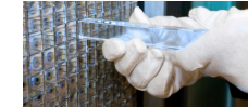
Insertion of lead tungstate crystals (over three times the density of conventional glasses) into the high granularity electromagnetic calorimeter of the ALICE detector giving percent scale energy measurements. (© CERN)
