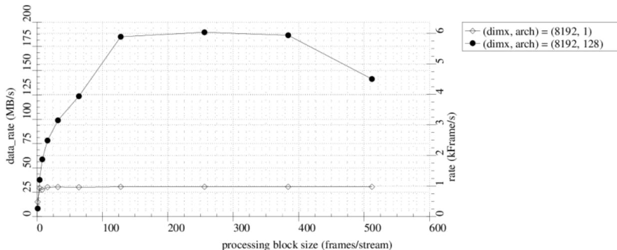
data rate (and frame rate) vs. 8kS frames per stream (1 str. on 128 cores in mode 10W) arch.=Nano
