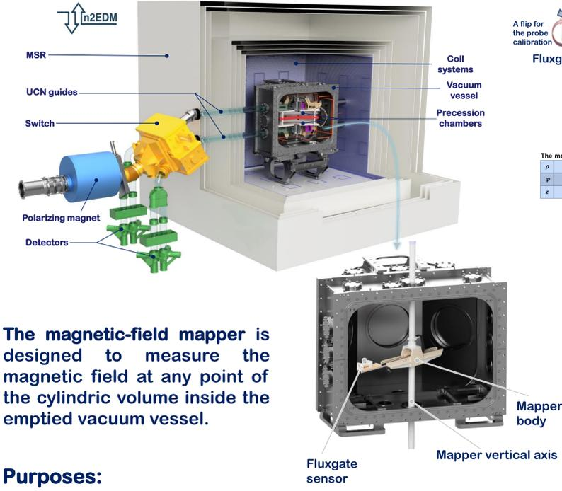
The magnetic-field mapper is designed to measure the magnetic field at any point of the cylindrical volume inside the emptied vacuum vessel.
