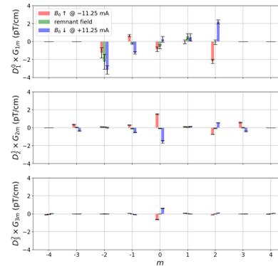
The bars at each l, m value correspond to the average normalized first-order gradient  $G_{l,m}$  of 6 mapping sequences. The error bars on each bar correspond to the reproducibility of the measurement.
