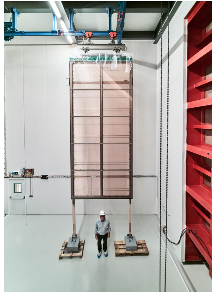
Anode Plane Assemblies (APA) - 6 m high x 2.3 m wide
