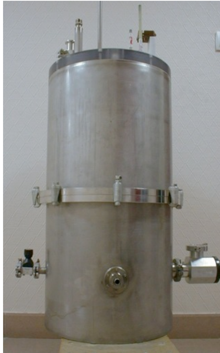
Cryostat with a thin hole made by the cryogenic team
