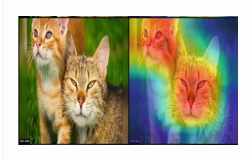
Grad CAM++ algorithm applied to a CNN. Colors represent filter activations. A hotter color means more emphasis was given on those pixels by the model.
