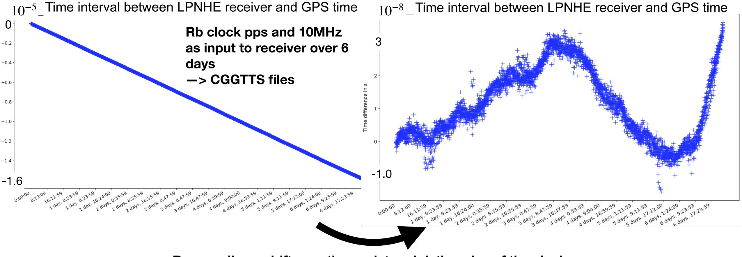
Remove linear drift over time = deterministic noise of the clock
