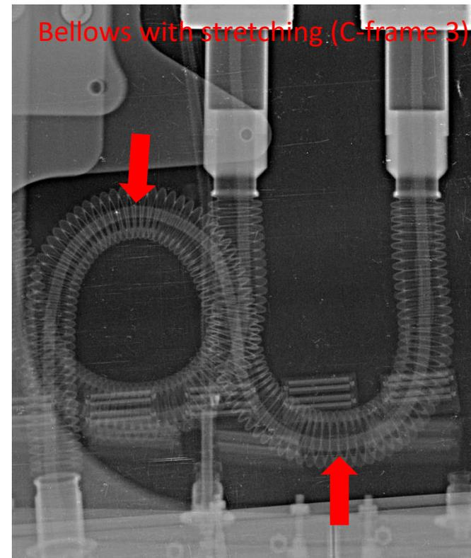
The bellows of a C-frame was then stretched to optimize the relative length and then X-rayed.
