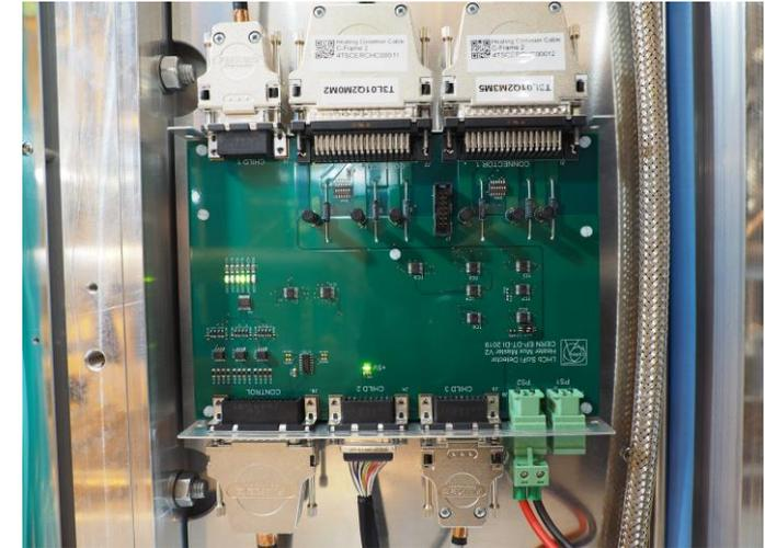
The full system of heating wires and temperature sensors, cables, boards etc. got integrated on the C-frame.
