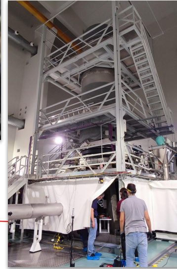
Virgo end tower and 42 kg suspended mirror
