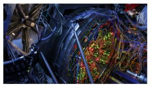
Fixed-target setup provides a high interaction probability, the detector features a large acceptance and high mass resolution.
