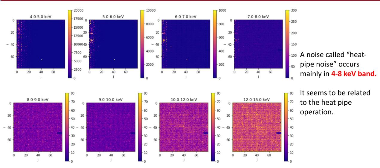
Shadowgrams integrated over the entire test period (without the radioactive source)
