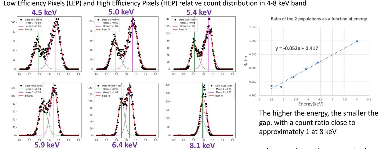
The CdTe pixels of ECLAIRs are made at two different periods (2008 and 2016). The detectors that count less come from the 2016 batch.
