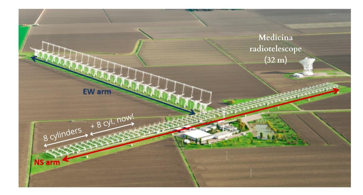
The focal line of 16 cylinders has been modified in order to group the signals of 64 dipoles together, providing 4 analogue signals per cylinder
