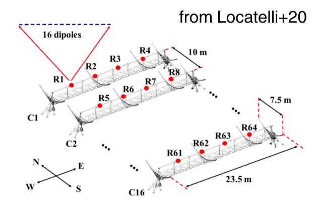
$u_0 = 408 \text{ MHz}$  BW = 16 MHz  $\Delta \nu_{ch} \simeq 14.5 \text{ kHz}$   $t_{samp} = 138 \ \mu s$
