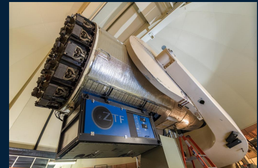
The Zwicky Transient Facility Camera (ZTF)
