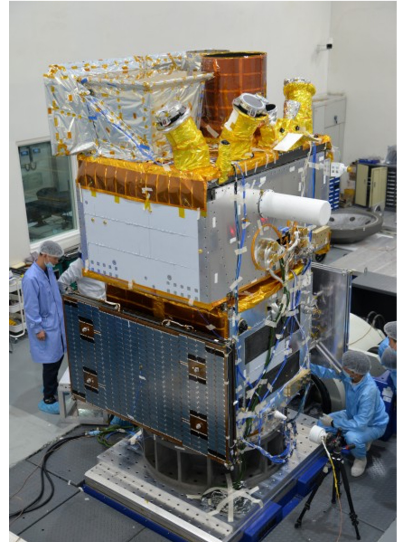
Qualification Model of SVOM satellite
