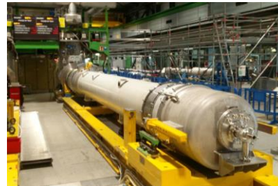
via HL-LHC technology 12 T Nb 3 Sn quadrupole
