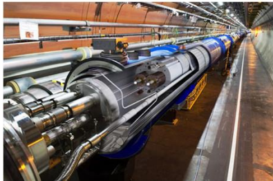
from LHC technology 8.3 T NbTi dipole
