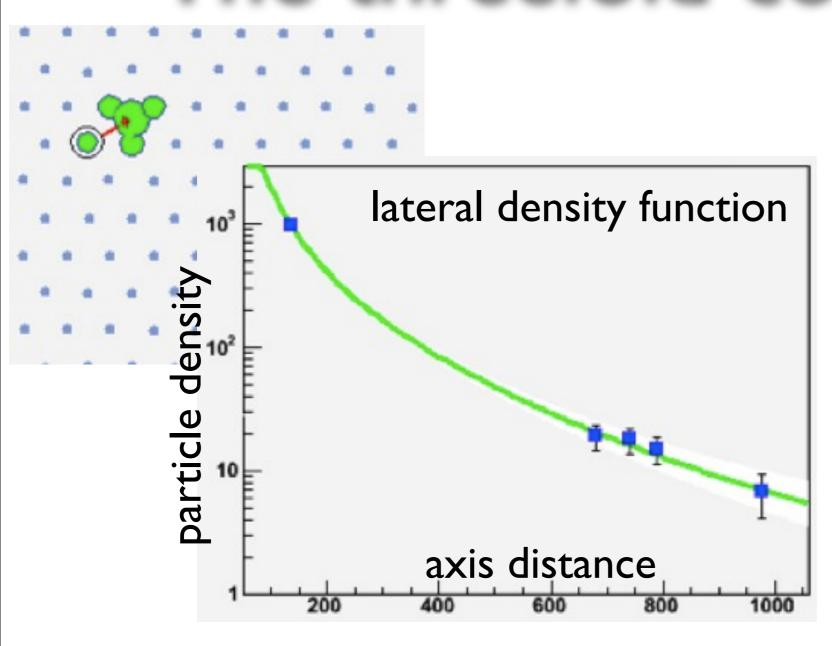
xcore =  $-8838 \pm 23$  m ycore =  $-3953 \pm 47$  m energy = 1.43 EeV (< 20%) axdist-A1 ~ 160 m axdist-A2 ~ 80 m axdist-A3 ~ 180 m
