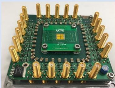
Hodoscope faisceau diamant CLARYS-UFT
