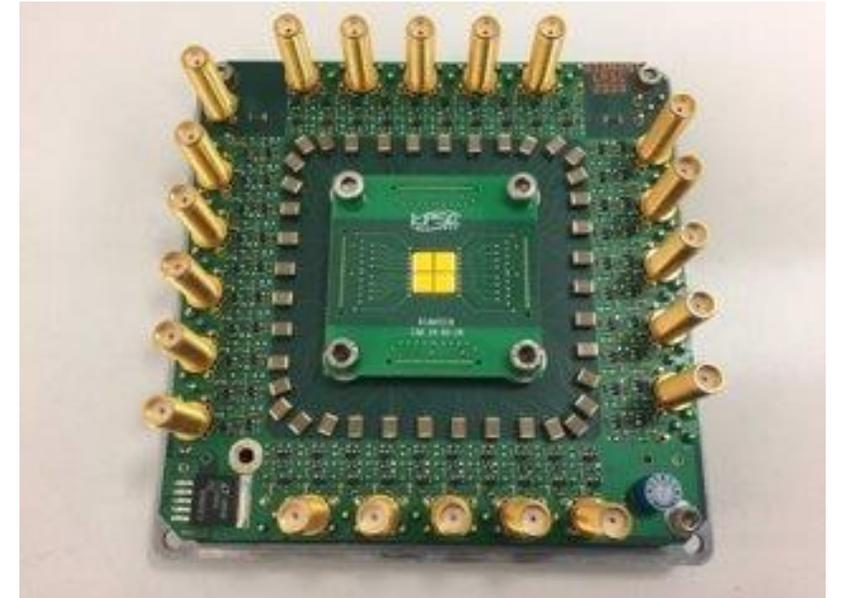
Prototype hodoscope CLaRyS
