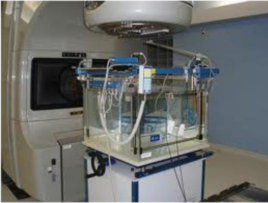
Motorized 3D water phantom equipped with IC or diodes system for dose distribution measurement
