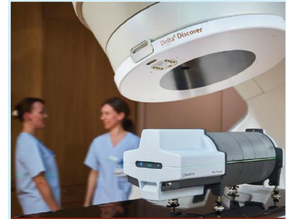
Delta4 phantom instrumented with 4040 diodes (5mm resolution at isocenter)
