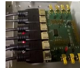
Acquisition module electronics MSP432P401R board with its daughter board for photodetection module interfacing
