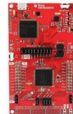
Acquisition module electronics MSP432P401R board with its daughter board for photodetection module interfacing
