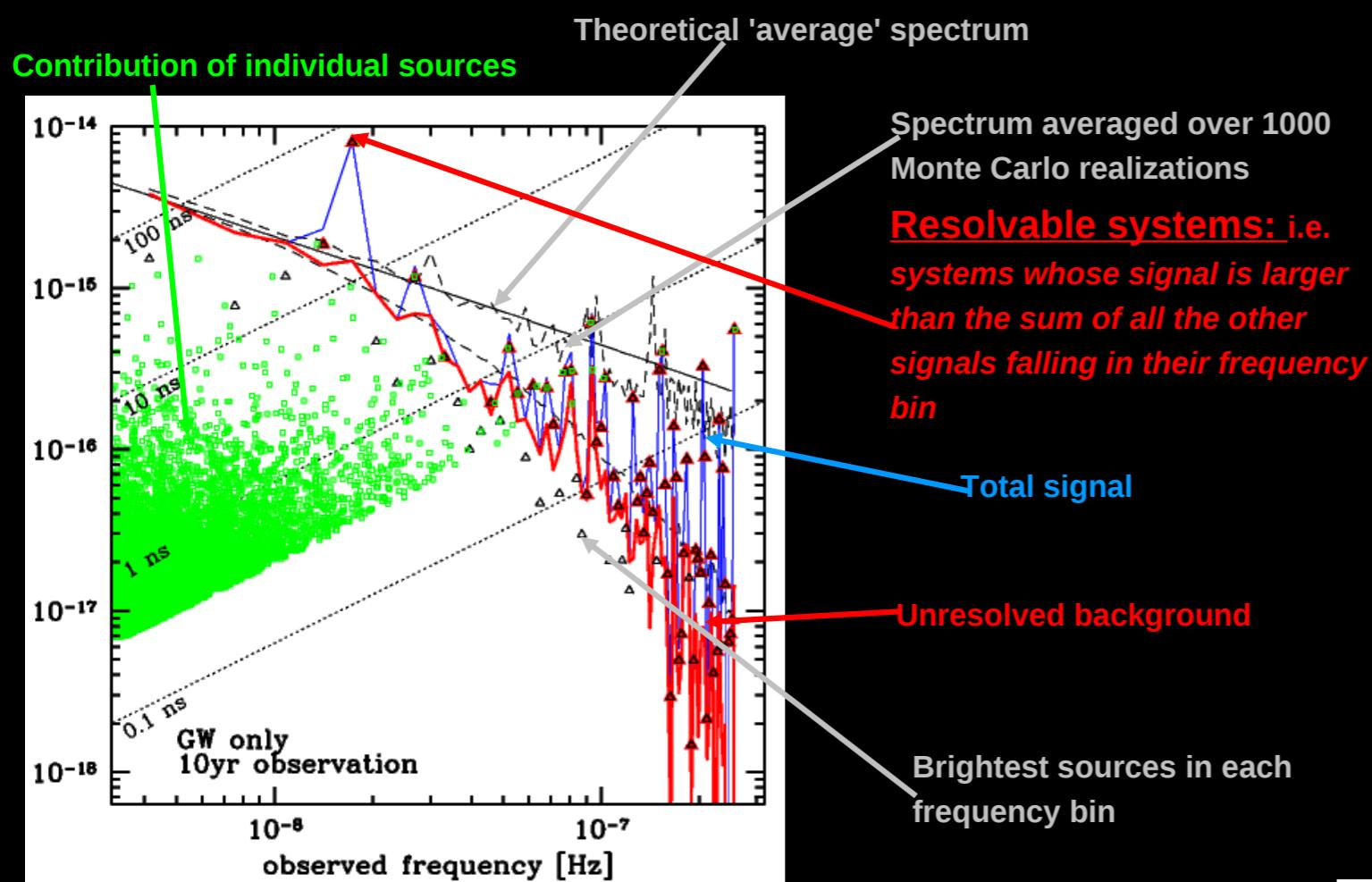
Superposition of multiple (overlapping) signals:
