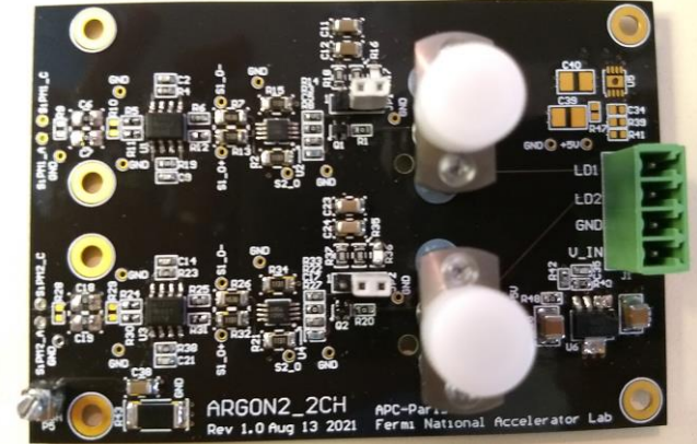
ARGON2x2 transmitter (collab w/Fermilab), installed in Coldbox1
