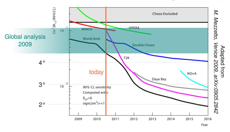
If combined analysis hints are confirmed by the present generation experiments (T2K and reactors), a  $\theta_{13} > 2-3^{\circ}$  measurement would allow to measure CP violation with next upgrades of already existing facilities
