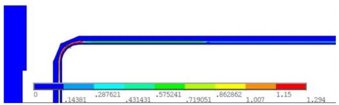
Maximum allowable water flow velocity in the water channel is taken to be 1 m/s (as recommended for heat exchangers)
