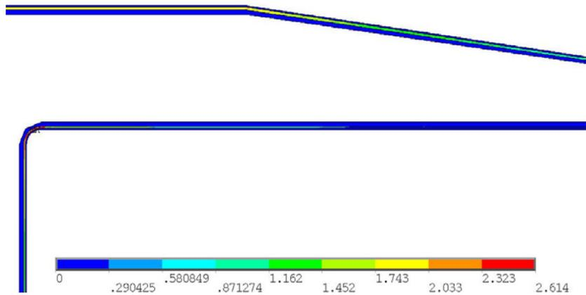
The flow rate now is locally 2.6 m/s. This flow rate is higher than the value recommended for flows in heat exchangers. It is possible to obtain the necessary flow rate by increasing the water channel gap (for this study it was assumed to be 2 mm)
