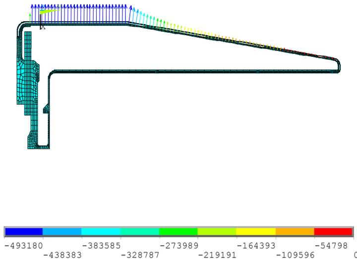
Magnetic pressure has been applied only to the horn inner conductor where it has the greatest effect. A rectangular pulse equivalent to the half-sine pulse has been used ( $p$  above is multiplied by  $2/\pi$ )
