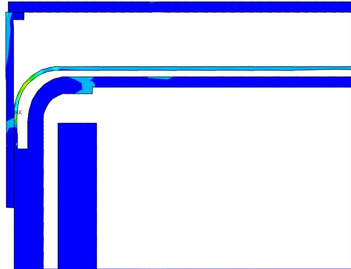
The equivalent (von Mises) stress is locally above 10 MPa. It stays below 10 MPa away from the region of localized stress.
