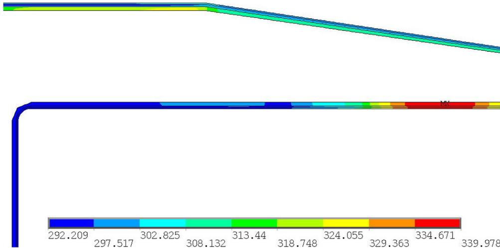
Maximum temperature is 340 K for the flow velocity of 1 m/s – this is acceptable for the present design, but no heat from the target has been taken into account. The efficiency of the target cooling system is being considered by B. Lepers
