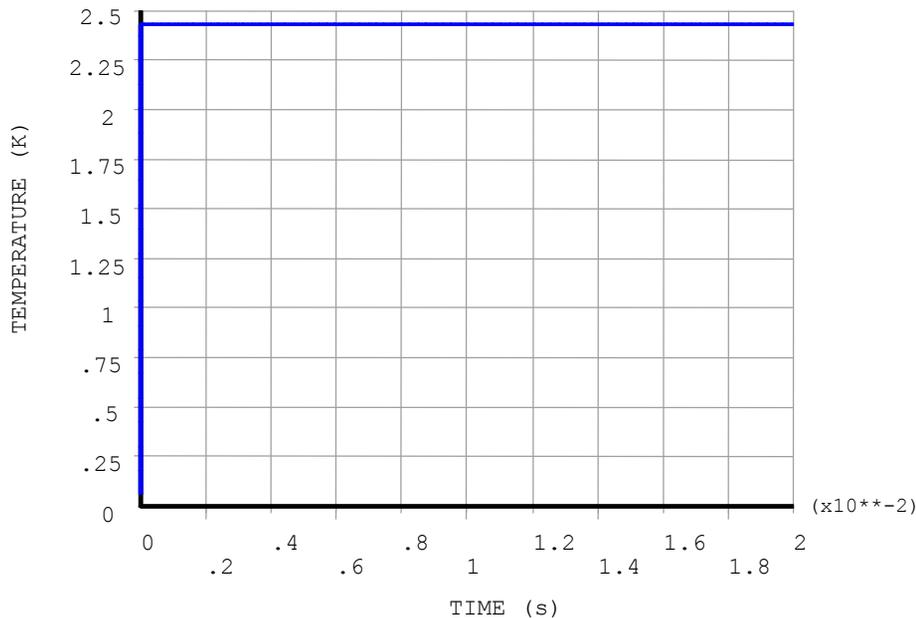
Temperature vs. time at a selected point on the horn waist (horn cylindrical part in the direct vicinity of the target).
