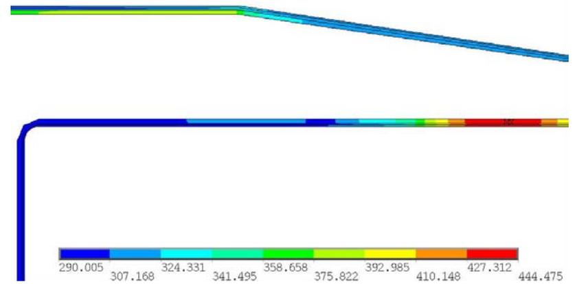
Maximum temperature of 446 K exceeds the design value for aluminium
