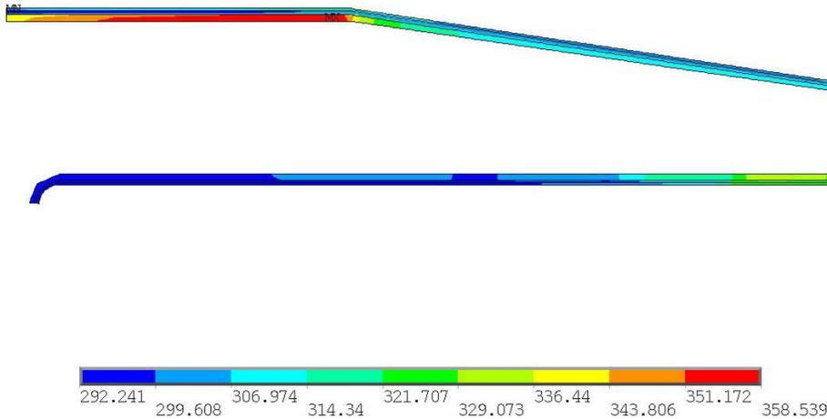
The maximum temperature on the horn goes down to 359 K
