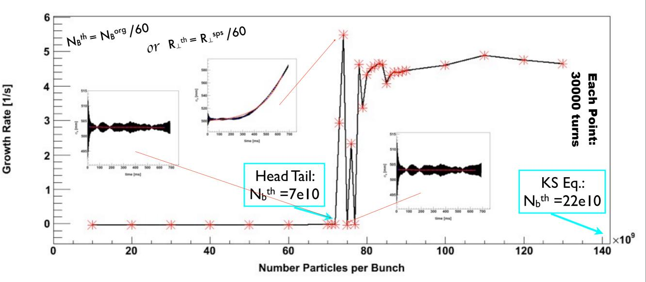
HeadTail indicates that for the current anticipated bunch intensity a 60 times smaller longitudinal shunt impedance than SPS is needed for the DR
