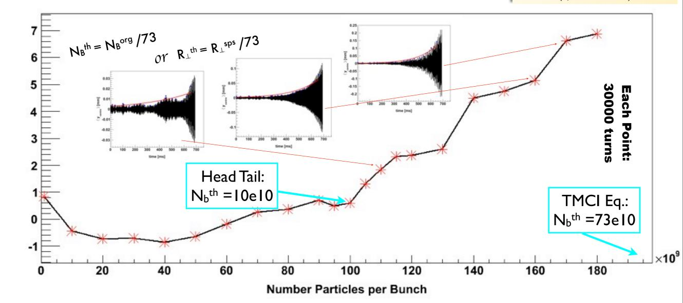
HeadTail indicates that for the current anticipated bunch intensity a 73 times smaller shunt impedance than SPS is needed for the DR
