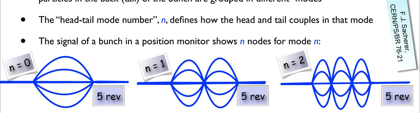
These head-tail modes in time domain can be Fourier transformed and squared to get the "head-tail power spectrum",  $h_n(\omega)$ :
