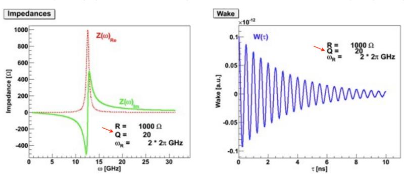
High Q → Narrow Band → Long Lasting Wake Field → Multi Bunch Instabilities
