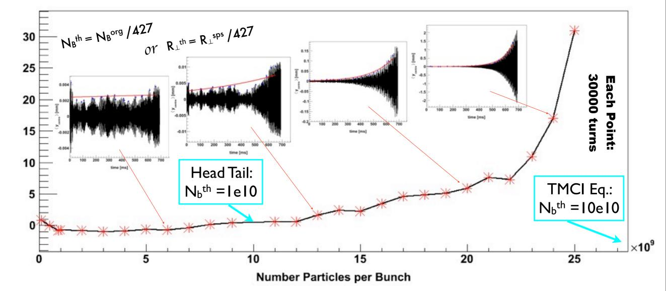
HeadTail indicates that for the current anticipated bunch intensity a 427 times smaller shunt impedance than SPS is needed for the DR
