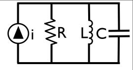
From the RLC circuit model we see the behavior of the resonant wake fields and the real and imaginary part of the impedance in the case of <u>high quality factor</u>; Narrow Band
