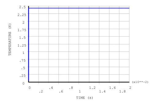
Temperature vs. time at a selected point on the horn waist (horn cylindrical part in the direct vicinity of the target).
