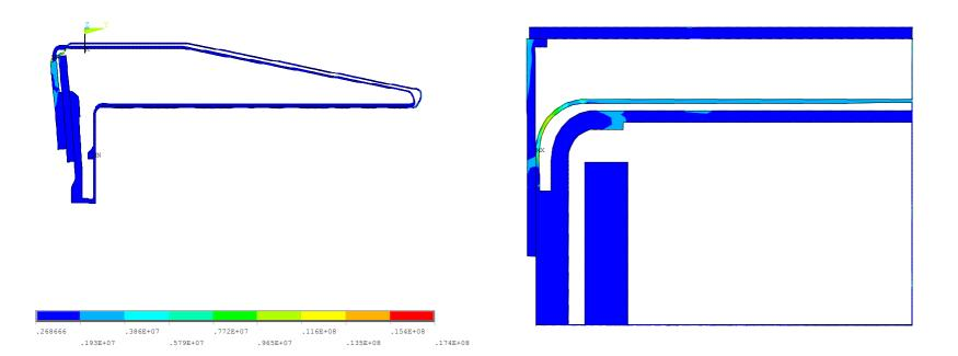
The equivalent (von Mises) stress is locally above 10 MPa. It stays below10MPa away from the region of localized stress.
