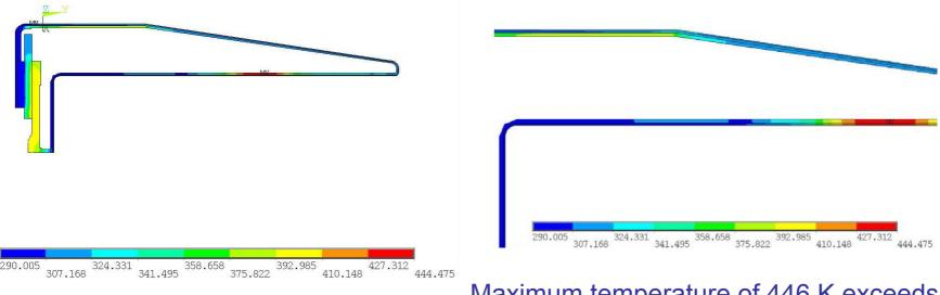
Maximum temperature of 446 K exceeds the design value for aluminium
