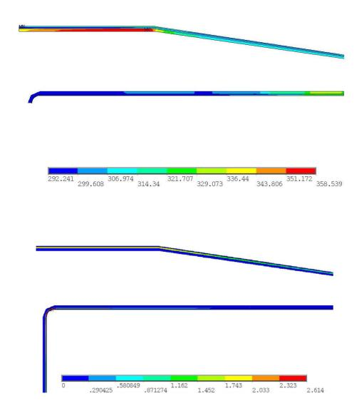
The maximum temperature on the horn goes down to 359 K
