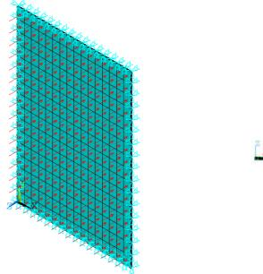
A simply-supported plate made of aluminium subjected to a pulse of heat flux applied to the top surface.
