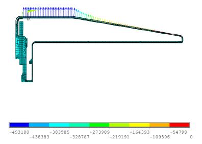
Magnetic pressure has been applied only to the horn inner conductor where it has the greatest effect. A rectangular pulse equivalent to the halfsign pulse has benn used (p above is multiplied by  $2/\pi$ )
