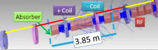
i.e. Doublet cell has the same components as the Singlet cell but the distance between coils of opposite polarity is not the same as the distance of same-polarity coils
