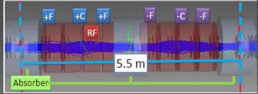
\*The Peak Electric Field was chosen such as to keep the energy of the reference particle constant, i.e. energy lost in absorbers=energy gained by RFs
