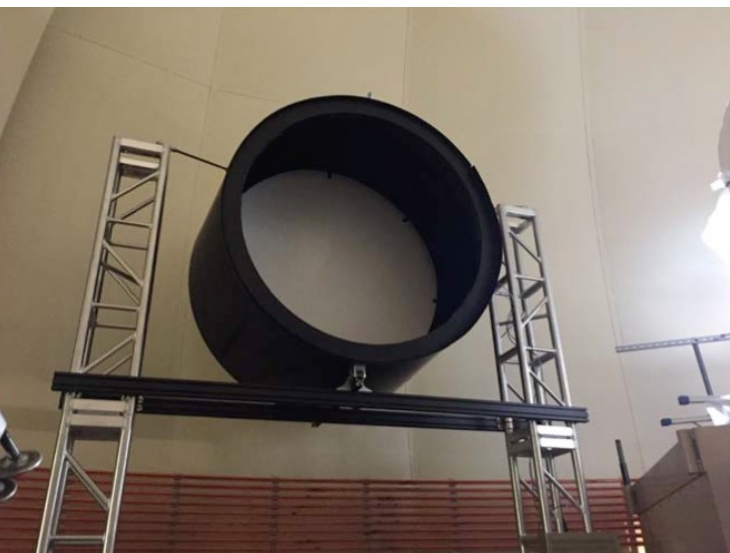
Flat-field illuminator (32 pulsed LEDs per colour)
