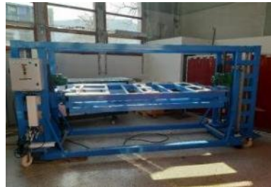
Handling and positioning tool for integration & tests
