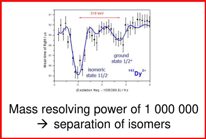
**Time of Flight Ion-Cyclotron-Resonance (TOF-ICR)**
