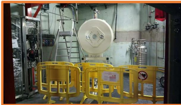
7 T superconducting magnet with 2 homogenous regions
