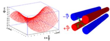
$$\Phi_0(t) = V_{DC} - V_{RF} \cos \Omega t$$
