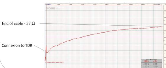
The first peak corresponds to the connection between TDR and cable. At the start of the measurement, the value measured is  $50 \Omega$  - the impedance of the cable. Then, the impedance increases up to the value of  $57 \Omega$ .
