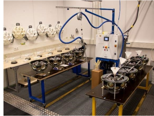
Pouring gel into the spheres
