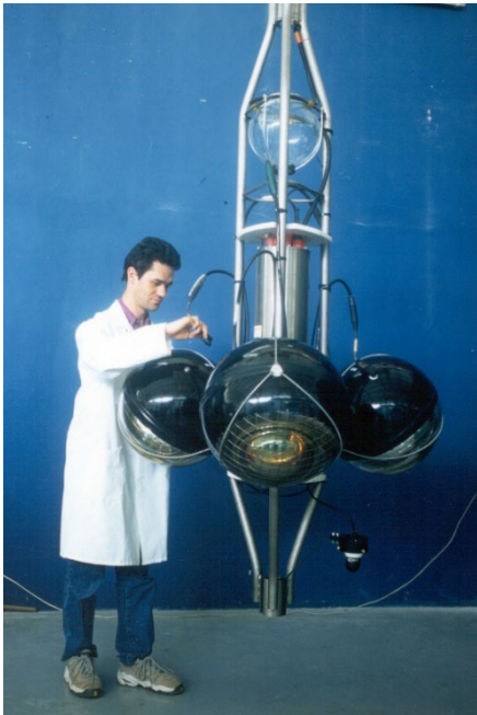
Assembly of one ANTARES 'storey'
