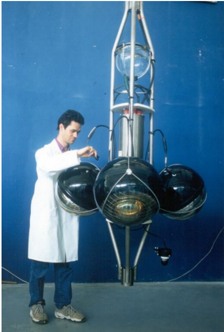
Assembly of one ANTARES 'storey'
