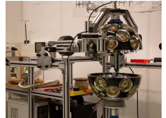
Sealing the sphere
