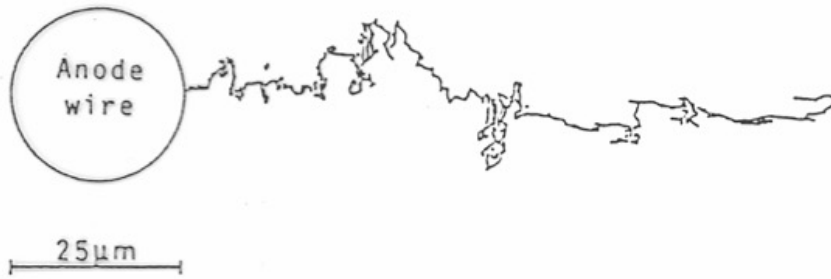
Fig. 5 Two dimensional display of a simulated drift process of one electron from starting point to anode wire surface.
