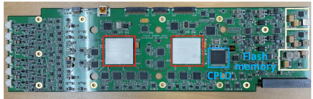
FAZIA / FEE(Front-End Electronics) new card
