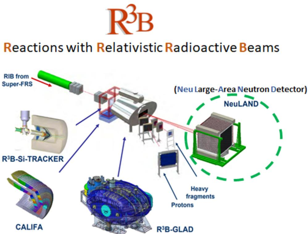
[Fig. 2] An illustration of the R3B setup. The NeuLAND is the modular neutron detection system that is used to detect outgoing neutrons from the reaction of the radioactive beam with the target.
