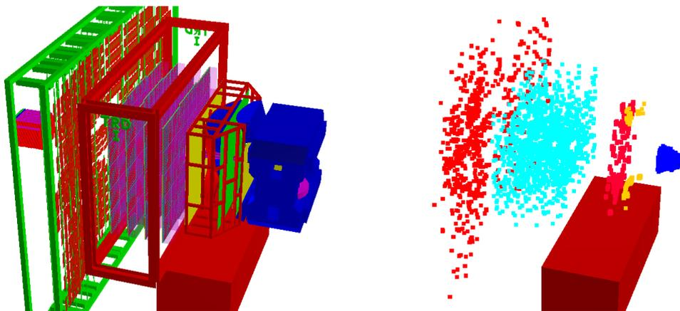
**[Fig.4]** Left shows the CBM simulation geometries for the future CBM experiment at FAIR. Consists of a blue magnet yoke on the right, followed by the RICH detector, the TRD, the TOF and PSD detector on the left. The beam enters from the right. The STS detector is contained inside the magnet. Right shows hits after transport from the demo scripts used during the DAC21 challenge.
