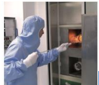
Annealing furnace in clean room environment
