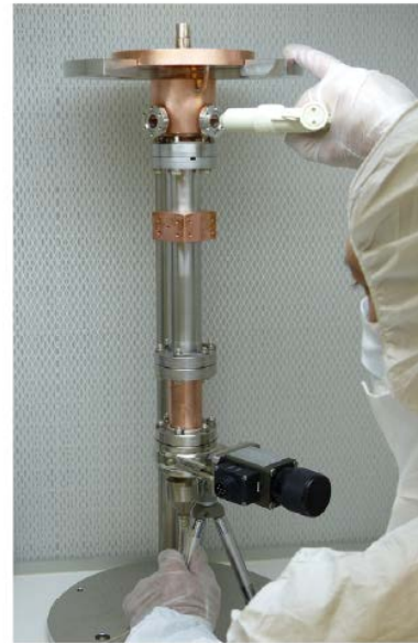
Fig. 2. Filtered N 2 blowing during the assembly of the coupler.
