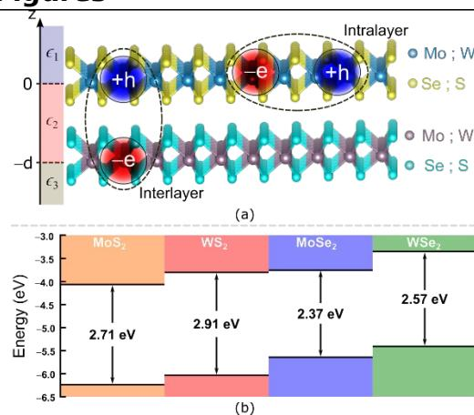
**Figure 1:** a) Schematic illustration of the double layered TMDs, separated by a spacer of dielectric constant  $\epsilon_2$  ( $-d \leq z \leq 0$ ) and width  $d$ , immersed in two materials of dielectric constants  $\epsilon_1$  ( $z > 0$ ) and  $\epsilon_3$  ( $z < -d$ ). This structure sustains both intralayer and interlayer excitons. (b) band alignment as measured from vacuum between the four TMDs considered in this work.
