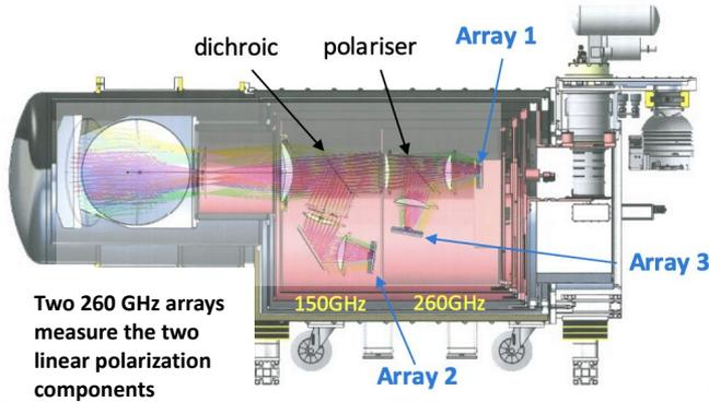
Two 260 GHz arrays measure the two linear polarization components
