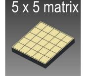
A possible detector design was simulated consisting of a  $5\times5$  matrix with a pitch of 1.9 mm (1850 µm pixel + 50 µm gap), performed by CNR-IMEM to obtain the best detector performances.
